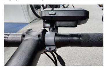
2.Use an Allen wrench to lock the console in the appropriate position on the bicycle
