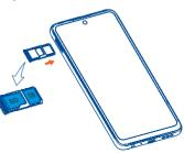
**NOTE:** A Verizon SIM card is already installed in your phone. This diagram shows SIM card location if you choose to remove or replace it.
