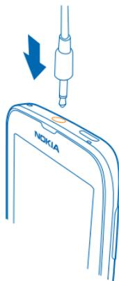
Do not connect products that create an output signal, as this may damage the device. Do not connect any voltage source to the audio connector. If you connect an external device or headset, other than those approved for use with this device, to the audio connector, pay special attention to volume levels.
