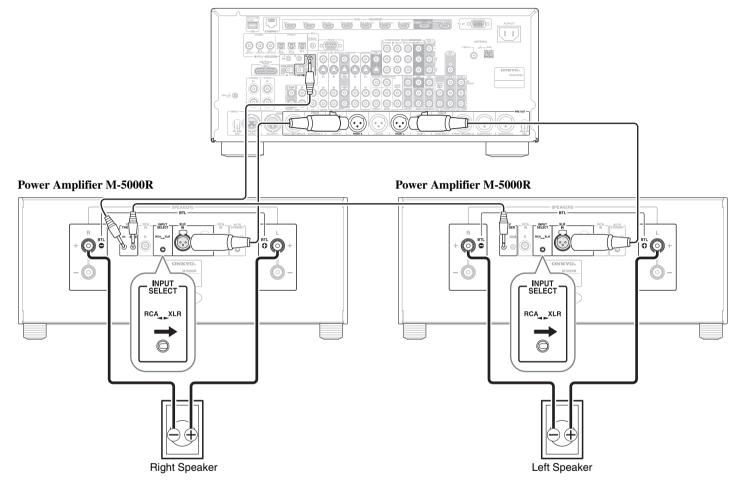
This is an example of the bridge connection with the AV controller PR-SC5508.
