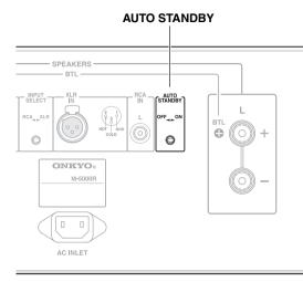
When **AUTO STANDBY** is turned **ON** side, the power amplifier will automatically enter Standby mode if the power amplifier receives no signal for 3 hours.
