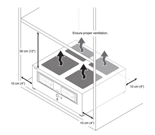
Install the power amplifier on a sturdy rack or shelf. Position it so that its weight is evenly dispersed on its four legs. Do not install the power amplifier in a place with vibration or an unstable location. The power amplifier is designed to have high conversion efficiency, however, its temperature will become much higher than other audio equipment. Therefore, make sure not to hamper heat dissipation by ensuring proper ventilation.
