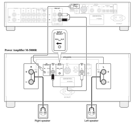
This is an example of the stereo connection using the preamplifier P-3000R.
