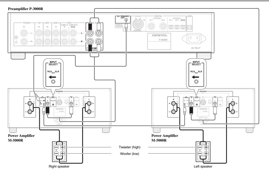
This is an example of the bi-amping connection using the preamplifier P-3000R.
