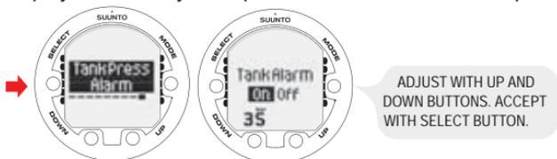
Three double beeps are also heard when the cylinder pressure goes down to the user-selected alarm pressure and when the remaining air time reaches zero.
