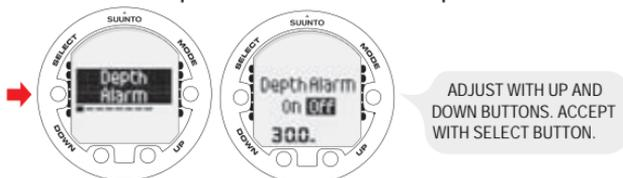
The depth alarm is factory-set to 30 m/131 ft, but you can adjust it according to your personal preference, or switch it off altogether. The depth range can be set from 3m to 100 m/9 ft to 328 ft.
