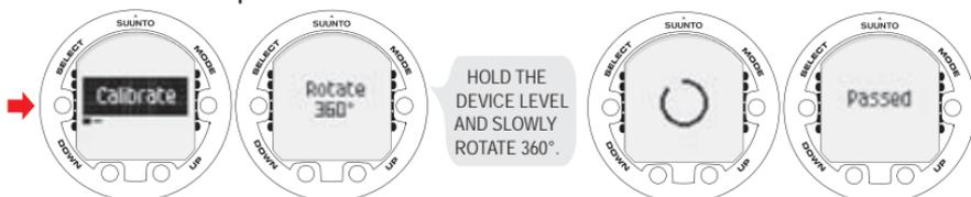
If the calibration fails several times in a row, it is possible that you are in an area with sources of magnetism, such as large metal objects, powerlines or electric appliances. Move to another location and try to calibrate the compass again. If the calibration continues to fail, contact an authorized Suunto service center.
