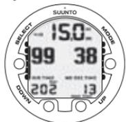
The change in your air consumption will be based on constant one second interval pressure measurements over 30 - 60 second periods. An increase in air consumption will influence the remaining air time rapidly, while a drop in air consumption will increase the air time slowly. In this way, an over optimistic air time estimation, caused by a temporary drop in air consumption, is avoided.
