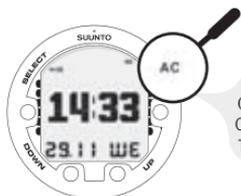
AC APPEARS IN THE TOP RIGHT CORNER OF THE DISPLAY, WHEN THE DIVE COMPUTER IS IN CONTACT WITH WATER. THIS ALSO ACTIVATES THE DIVE MODE.
