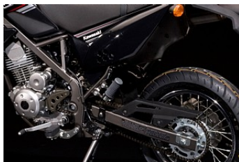
Highly rigid perimeter frame purpose-built for the 125 cm 3 class
