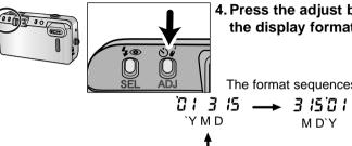
4. Press the adjust button to change the display format.
