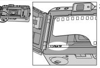
2. Place the film cartridge into the film chamber. Extend the film leader to the "FILM TIP" mark, making sure it lays flat.
