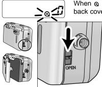
When **o** blinks on the data panel, open the back cover and remove the film.
