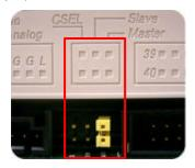
Note: Installing jumper pins besides the ones for device configuration settings may be the cause of damage or abnormal drive operation.
