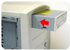
6. Use four provided screws (size: M3x0.5x4mm) to secure the drive into the half-height bay. The screws electronically ground the drive.
