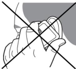
The antenna is integrated in your phone, under the back cover at the top. Avoid putting your fingers on this area when the phone is switched ON. If your fingers obstruct the antenna, the phone may have to operate with a higher power level than usual; decreasing its efficiency quickly. It could also affect the quality of your communications.
