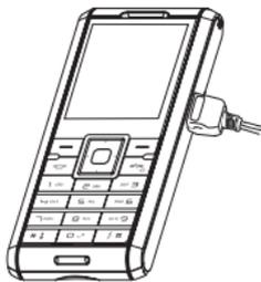
Your phone is powered by a rechargeable battery. A new battery must be charged for 4 hours at least before being used for the first time. It reaches its optimum capacity after a few cycles of use.
