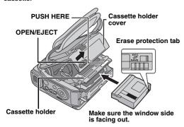
1 Slide and hold **OPEN/EJECT** in the direction of the arrow, then pull the cassette holder cover open until it locks. The cassette holder opens automatically.
