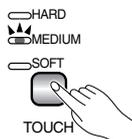
To select a touch sensitivity type press the [TOUCH] button a few times until the indicator corresponding to the desired type lights (the indicators light in sequence each time the [TOUCH] button is pressed).
