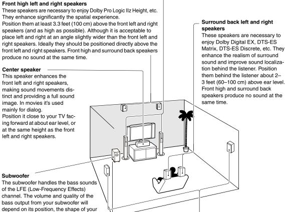
listening room, and your listening position. In general, a good bass sound can be obtained by installing the subwoofer in a front corner, or at one-third the width of the wall, as shown.
