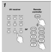
Use the AV receiver's input selector buttons to select the input source.
