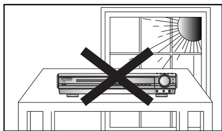
Do not expose the unit to direct sunlight or other heat sources. This could lead to overheating and malfunction of the unit.
