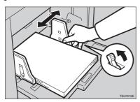
When you finish printing, shift the feed roller pressure lever to the Standard paper position.
