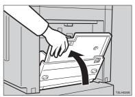
Move the end plate until the plate handle is flush with the end of the tray.
