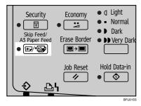
Use the [▲][▼]keys to select Skip Feed, and then press the [OK] key.
