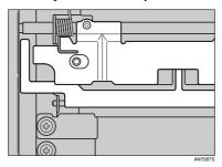
1 Insert the drum until it locks into position, and then lower the lock lever.
