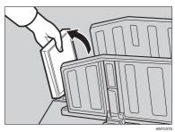
Lift the paper delivery end plate and adjust it to match the paper size.
