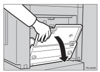
Shift the paper feed side plates lock lever forward. Adjust the side plates to match the paper size.
