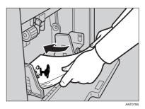
Exchange the drum unit. See p.65 "Changing the Colour Drum Unit".
