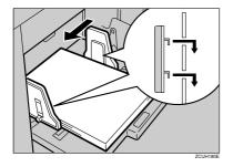
Shift the lock lever to its original position.
