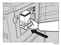
**1** Lower the drum unit lock lever.
