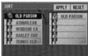
**5b** The Today's Plan list with the new sequence is displayed. If the sequence displayed is acceptable, select "APPLY" and press ENTER. If the new sequence displayed is unacceptable, you can reinstate the original sequence by selecting "RESET" and pressing ENTER.
