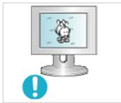
▶ When using a fixed screen for a long time, an afterimage or stain may occur.
