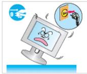
▶ When you drop the product or the case is broken, turn the power off and disconnect the power cord. Contact a Service Center.
