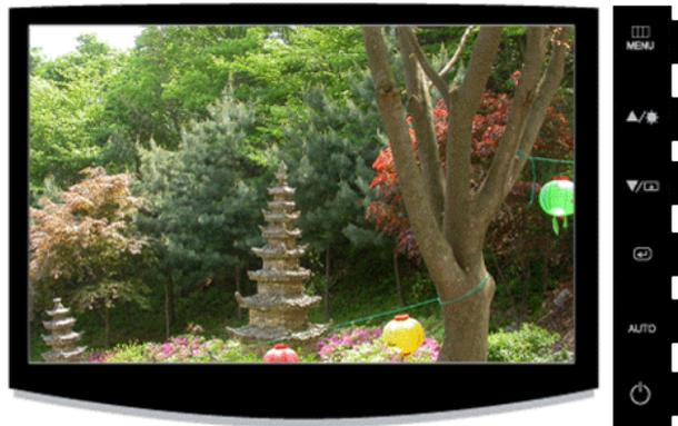
When OSD is not on the screen, push the **Brightness** (
