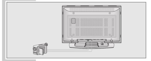
Connect the yellow socket »AV IN VIDEO« on the television and the corresponding socket on the camcorder (VHS, Video 8) with a cinch cable (picture signal);
