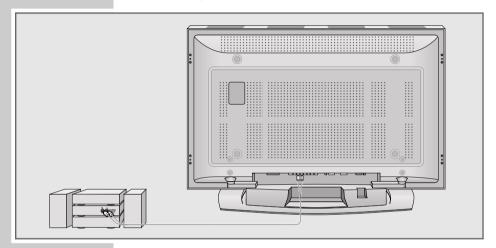
Connect the white and red sockets »AV OUT L R « on the television and the corresponding sockets on the HiFi with a cinch cable.
