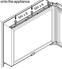
4. Slide the appliance into the recess leaving a 21 mm gap between the body of the unit and the front face of the door.
