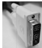
DVI-D connector of DVI-D monitor
