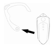
Flip the ear clamp over, and snap it back onto the headset by applying gentle pressure on the base of the ear clamp ring.
