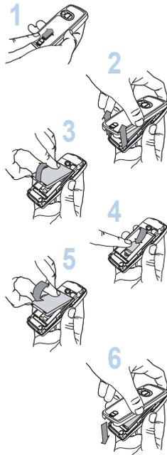
The SIM card is inserted under the phone's battery. Ensure that the phone is switched off and the charger disconnected.
