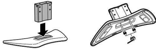
**3** Insert the stand into the opening on the bottom of the TV.
