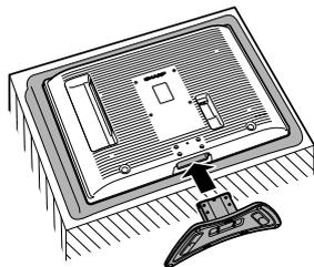
**4** Insert and tighten the 4 long screws on the rear of the TV as shown.
