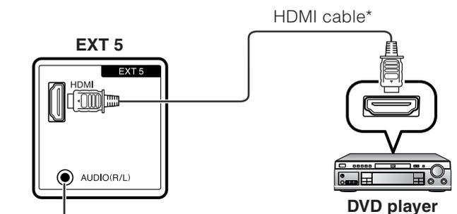
When using an HDMI-DVI conversion adapter/cable, input the Audio signal here.
