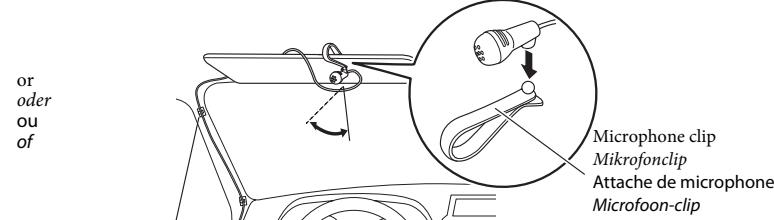
We recommend to attach the microphone near the steering wheel using the microphone holder.
