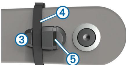
The pedal magnet must be within 5 mm of the GSC 10. The indication line ⑤ on the pedal magnet must line up with the indication line ⑥ on the GSC 10.
