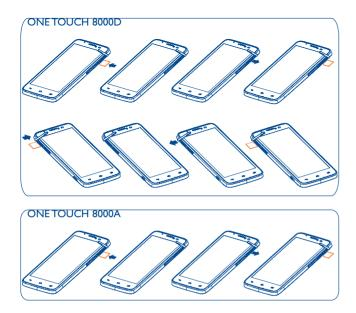
To install, place the SIM card chip facing downwards, and then slide it into its slot. Make sure that it is correctly inserted. To remove the card, press and slide it out.
