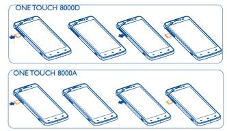
Insert the microSD card with golden contact facing downwards into the slot. To remove the microSD card, gently press and slide it out.
