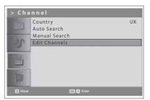
Analog channels are editable only in **Analog TV** input mode. Please make sure the main Input is set to **Analog TV** using **TV/AV** button.
