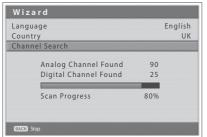
When you turn on your TV for the first time after purchase or perform the default setting, the initial setup wizard will appear automatically. You can easily setup the available analog and digital channels using the wizard.
