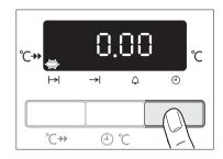
3. Using the +/- control knob set the desired cooking time.
