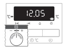
After approx. 5 seconds, the flashing stops and the clock displays the time of day set.
