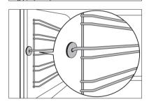
To re-insert, first hook the rail into place at the back (1) and then insert the front and press into place (2).
