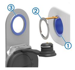
Make sure the pedal pod mounting face ③ contacts the crank arm only at its mounting face (or the washer used to fill the recess).
