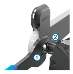
**NOTE:** The spindle and crank for the left pedal has a left-handed (reverse) thread.
