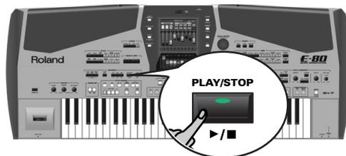
The Recorder now counts in one measure, after which recording starts.
