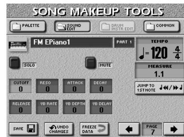
Press the field of the parameter you want to edit and use the **[DATA/ENTRY]** dial or the **[DEC]/[INC]** buttons to set the desired value. You can also press the **[DATA/ENTRY]** dial and use the numeric pad.
