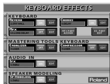
On this page, you can switch the REVERB, CHORUS and MFX processors on and off by pressing their **[OFF/ON]** button icons to the right of their "display". If you only need another reverb type, press the REVERB display and use the **[DATA/ENTRY]** dial or the **[DEC]/[INC]** buttons to select it. If you also need to change certain aspects of that effect...
