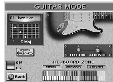
The [Off/On] switch icon allows you to switch the Guitar mode on or off. If you selected this page by pressing EASY SETTING [GUITAR], it is already set to on.
