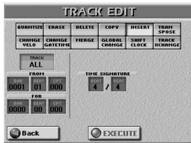
INSERT allows you to insert space and shift data that lie behind the FROM position further towards the end of the song (this is the exact opposite of DELETE). These empty measures can be "filled" using the COPY function or by recording new phrases in that area (using PUNCH IN/OUT, for example, page 183).
