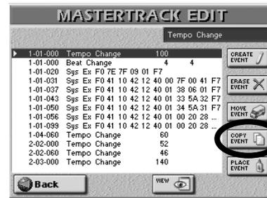
**Note:** For this function, you could take advantage of the VIEW filter to avoid selecting event types that should not be included in the copy. See "VIEW" on p. 191.
