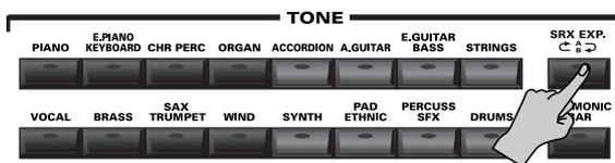
Press it once to select the expansion board in slot "A", or twice to select the board in slot "B". If your E-80 only contains one board, the other slot cannot be selected. (It is perfectly possible to connect that board to slot "B" and to leave slot "A" empty.)
