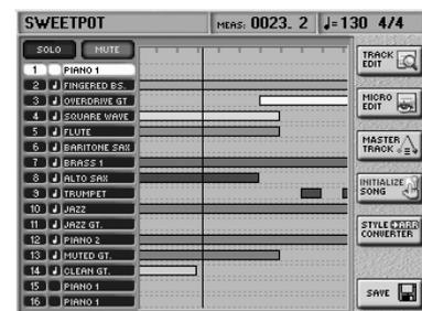
The "MEAS" field at the top of the display informs you about the current measure. The tempo and time signature are displayed next to it. Use the RECORDER **◀** and **▶** buttons to jump to another measure or **TOP I** to return to the beginning of the song.
