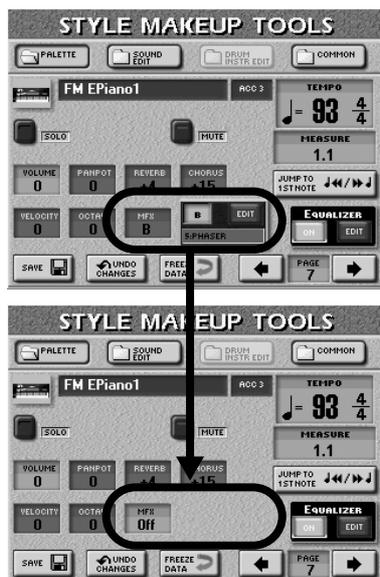
If you select “A”, “B” or “C”, an additional display and an **[EDIT]** button icon appear. The display shows the name of the effect type currently assigned to the selected MFX processor.
