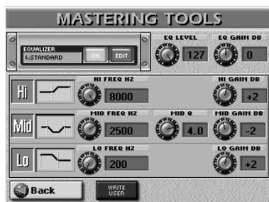
The equalizer has the same function as the BASS, MID and TREBLE knobs on an amplifier: it allows you to color the sound or to apply tonal corrections that help you avoid saturating the speakers.
