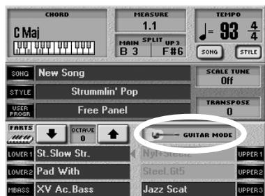
The UPPER1 field below "GUITAR MODE" shows the name of the currently selected guitar sound. You cannot select other guitar sounds for UPPER 1 simply by pressing this field: press the "GUITAR MODE" field to jump to the page shown above, then change the settings you don't like. (UPPER2's guitar sound is assigned automatically and can never be changed.)
