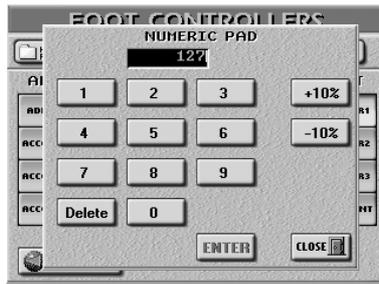
Enter the value you want to use, then press the **[ENTER]** field. If necessary, you can use the **[Delete]** field to correct erroneous entries before pressing **[ENTER]**.
