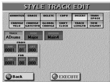
INSERT allows you to insert space and shift data that lie behind the FROM position further towards the end of the track (this is the exact opposite of DELETE). The empty measures you create can be "filled" using the COPY function or by recording new phrases in that area.
