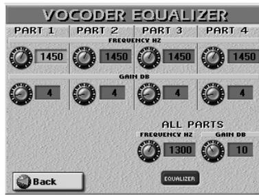
This page contains a simple equalizer for each Vocoder part, as well as an EQ band that applies to all four voices simultaneously, for added flexibility. These are connected in series.
