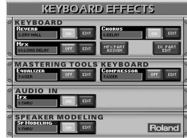
On this page, you can switch the AUDIO IN IFX processor on and off by pressing the **[OFF/ON]** button icon to the right of its "display".
