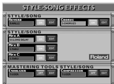
On this page, you can switch the REVERB, CHORUS and/or three effects processors off by pressing the **[OFF/ON]** button icon to the right of their "displays".
