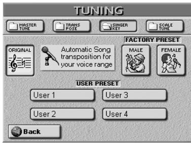
This page contains three presets: **ORIGINAL** means that the song is not transposed, while **MALE** and **FEMALE** adapt the song's key to the "typical" range of a male or female voice.
