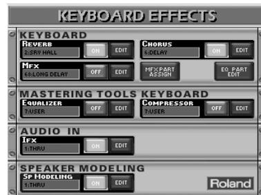
On this page, you can switch the **SPEAKER MODELING** processor on and off by pressing the **[OFF/ON]** button icon to the right of its "display".
