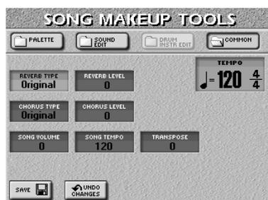
Press the field of the parameter you want to edit and use the **[DATA/ENTRY]** dial or the **[DEC]/[INC]** buttons to set the desired value.
