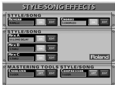
On this page, you can switch the REVERB, CHORUS and/or three effects processors off by pressing the **[OFF/ON]** button icon to the right of their "displays". If you only need to select another effect type, press the REVERB, CHORUS or an MFX A~C display and use the **[DATA/ENTRY]** dial or the **[DEC]/[INC]** buttons to select the algorithm. If you also need to change certain aspects of that effect...
