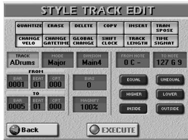
The CHANGE VELO function allows you to modify the dynamics (called "velocity") of a track or excerpt. See p. 185 for details. Only note events can be changed.
