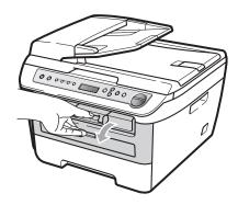
Slowly take out the drum unit and toner cartridge assembly. The jammed paper will be pulled out with the toner cartridge and drum unit assembly.
