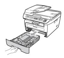
While pressing the green paper guide release lever, slide the paper guides to fit the paper size. Make sure that the guides are firmly in the slots.
