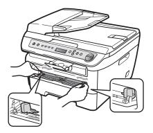
4 Using both hands, put one sheet of paper or one transparency in the manual feed slot until the front edge touches the paper feed roller. When you feel the machine pull in the paper, let go.
