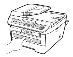
3 Using both hands, slide the manual feed slot paper guides to the width of the paper that you are going to use.
