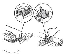
3 Put paper in the tray, and make sure that the paper is below the maximum paper mark (1). The side to be printed on must be face down.
