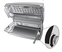
**8** Close the device. Insert the paper tray in the opening provided for it behind the paper feeder. Insert paper again.
