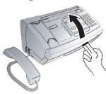
Lock the cover of the machine completely into place when opening the machine. You could be injured if the cover falls while you are working on the machine.
