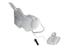
We recommend direct connection to the machine because this allows the fax switch to function optimally and to control the additional devices.
