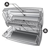
6 Close the scanner cover and the cover of the automatic document feeder. Both the supports must securely snap into place. **7** Turn the blue gear wheel forward to tension the ink film. The ink film must not have any creases.
