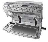
4 Remove both the rolls from the device. The used ink film cannot be reused.
