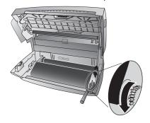
7 Close the device. Insert the paper tray in the opening provided for it behind the paper feeder. Insert paper again.
