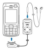
To control the music player, use the media keys of the remote control unit. To adjust the earpiece volume, press the volume key on the side of the remote control unit. To lock the remote control keys, slide the lock switch on the side of the remote control unit.
