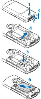
Use only compatible Reduced Size MultiMediaCards (RS-MMC) with this device. Other memory cards, such as Secure Digital (SD) cards, do not fit in the memory card slot and are not compatible with this device. Using an incompatible memory card may damage the memory card as well as the device, and data stored on the incompatible card may be corrupted.
