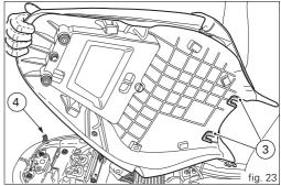
The helmet hook (4, fig. 23 - fig. 24) for attachment of the rider's and passenger's helmets is located on the rear of the frame under the seat. Pass the cable through the helmets and insert the end of the cable in the catch; leave the helmets hanging and replace the seat to secure them.
