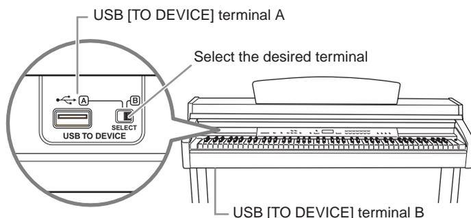
Both are the same terminal; however, both cannot be used at the same time. Use the **[SELECT]** switch to select the desired terminal. Switching to "A" selects the terminal on the left of the panel, while switching to "B" selects the terminal panel at the bottom. When the device is mounting, the FILE "LOAD" indicator flashes. When the mounting operation is completed, the indicator goes off.
