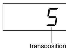
The [TRANPOSE] button indicator remains lit when a transposition setting other than “0” is selected. Every time the [TRANPOSE] button is pressed after that switches the transposition function ON or OFF.
