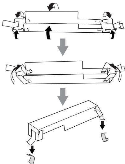
**3-2** Cover the top of D and E with the side panel protection pad. Then, fix the protection pad with the adhesive tape.
