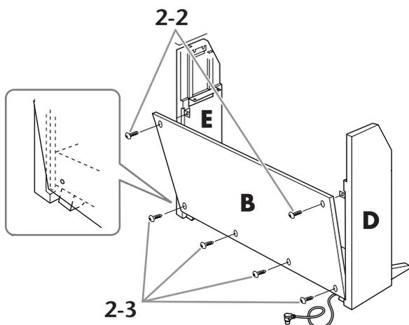
**2-3** Temporarily secure the bottom part using four 4 x 20 mm tapping screws.
