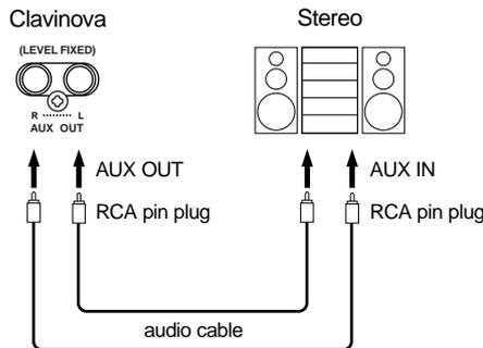
When these are connected (with RCA pin plug; LEVEL FIXED), the sound is output to the external device at a fixed level, regardless of the [MASTER VOLUME] slider setting.
