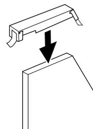
**3-3** Align the dimple on side A with the inner side of D and E. Simultaneously lower the left and right side of A, and secure with D and E.
