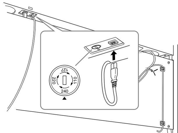
Insert the AC power cord plug into the AC INLET.
