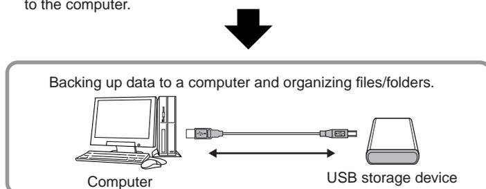
**■ Copying files from a computer hard disk to a USB storage device**
