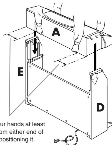
**3-4** Support the backside of D and E with your hand, and slightly push A in from the keyboard side until it stops.
