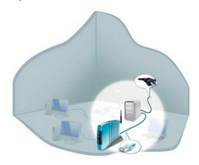
Use a wired connection to connect your home server to your broadband router or to a switch that is connected to your broadband router. Then connect your home server to an electrical outlet.
