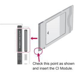
the module is not inserted properly, this can cause damage to the TV and the
