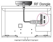
3 Attach the RF Dongle to the velcro as shown below and then turn on the TV.
