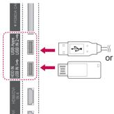
To disconnect a USB storage device, make sure to end the connection properly to prevent damages to the TV or files.
