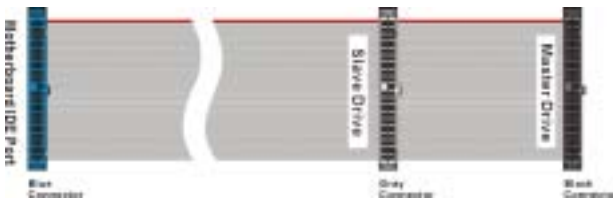
Figure 2-10. Ultra DMA 66 Ribbon Cable Outline
