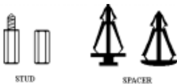
Figure 2-1. The outline of stud and spacer
