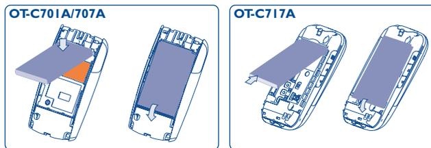
Insert and click the battery into place, then close the telephone cover.
