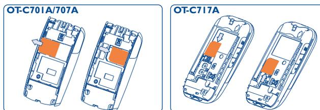
Place the SIM card with the chip facing downwards and slide it into its housing. Make sure that it is correctly inserted. To remove the card, press it and slide it out.
