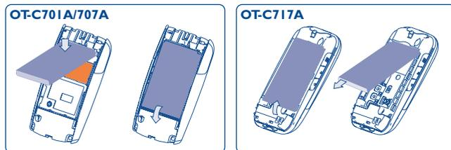
Unclip the cover, then remove the battery.
