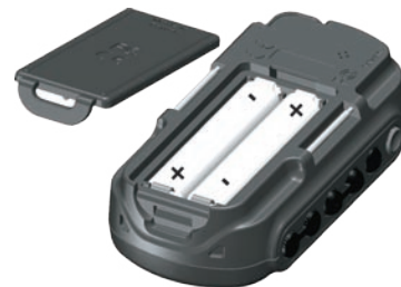
Installing AAA batteries into the Foretrex 101
