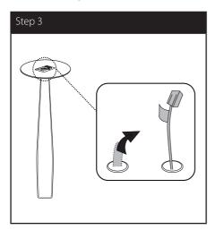
4. Insert the connector to the bottom of the base. Connect the speaker wire to the terminal on the base.
