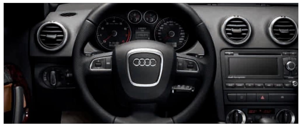
3-spoke multi-function steering wheel with gear-change controls
