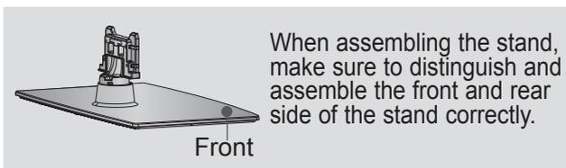
When assembling the stand, make sure to distinguish and assemble the front and rear side of the stand correctly.
