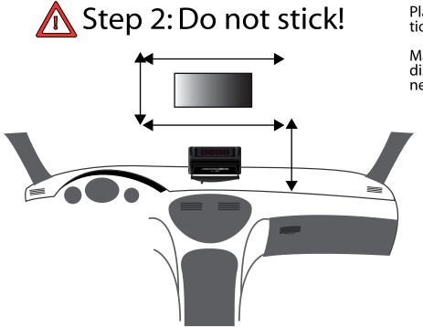
Place the reflector on the windshield - without removing the protection! - and check the position of both the unit and the reflector.
