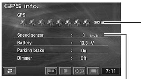
Blinks when the Speed Pulse signal is being input.
