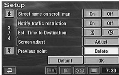
**3** Tilt the joystick to select “Delete” under “Previous point” and press ENTER.
