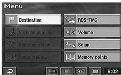
**Ex.3** Search for a desired destination by scrolling the map with the joystick. The map scrolls in the direction in which the joystick is tilted. Bring the destination point on the map under the reticule icon and press ENTER. The point setting menu appears.
