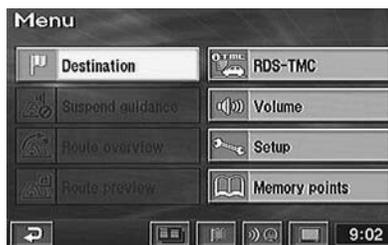
**Ex.2** Select (highlight) “Destination” from the main menu by tilting the joystick on the remote control and press the ENTER button on the top of the joystick.
