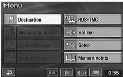
**4** The display shows the sub-menu for the selected main menu item. Highlight (select) a desired sub-menu item by tilting the joystick and press the ENTER button.
