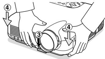
4. Lower the front of the projector to the desired height and release the Adjustable Tilt Foot Lever to lock the Adjustable tilt foot. There is approximately 7 degrees of up and down adjustment for the front of the projector.
