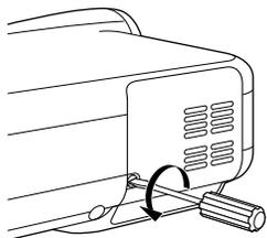
2. Loosen the two screws securing the lamp housing until the screwdriver goes into a free-wheeling condition. The two screws are not removable.
