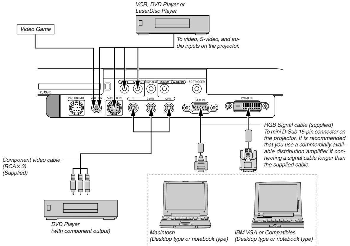
**NOTE:** When using with a notebook PC, be sure to connect between the projector and the notebook PC before turning on the power to the notebook PC. In most cases signal cannot be output from RGB output unless the notebook PC is turned on after connecting with the projector.
