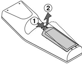
2. Remove both old batteries and install new ones (AA). Ensure that you have the batteries' polarity (+/-) aligned correctly.
