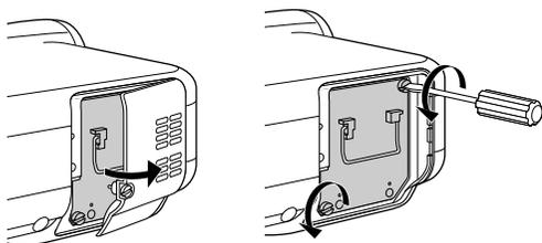
3. Remove the lamp housing by pulling out the handle.
