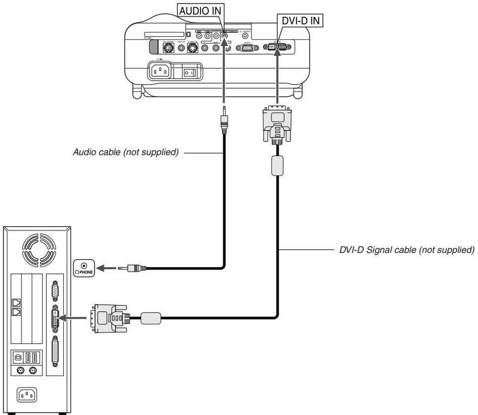
To project a DVI digital signal, be sure to connect the PC and the projector using a DVI-D signal cable (not supplied) before turning on your PC or projector. Turn on the projector first and select DVI (DIGITAL) from the source menu before turning on your PC.
