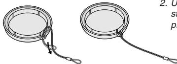
2. Use the rivet to attach the string to the bottom of the projector.
