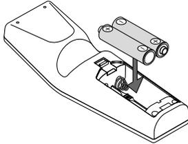
3. Slip the cover back over the batteries until it snaps into place. Do not mix different types of batteries or new and old batteries.
