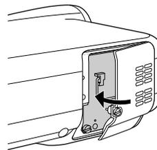
7. Tighten the lamp cover screw. Be sure to tighten the screw.
