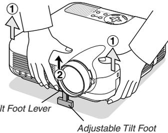
2. Push up the Adjustable Tilt Foot Lever on the front of the projector to extend the adjustable tilt foot (maximum height).
