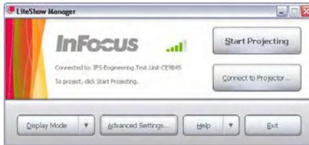
signal strength is gray bars when no wireless network is connected, green bars when connected. adjust the antenna angle on the back of the adapter to maximize wireless signal strength.
