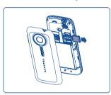
Unclip the back cover and gently push the memory card until unlocked. Take out your MicroSD card and clip the back cover.
