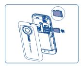
Unclip the back cover and insert the MicroSD card into the slot.
