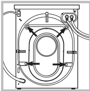
3. Remove the four protective screws and the rubber bush with the respective spacer, situated on the rear of the appliance (see also the installation leaflet). **NB:** The plastic spacers may fall down inside the machine once the bolt
