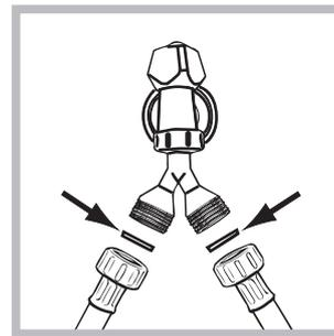
1. Connect the supply pipe to the water mains, fitting the rubber gasket and the filter supplied with the appliance and ensuring that they are firmly tightened to the taps.
