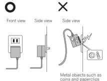
Connect the AC adaptor into a wall socket. Only connect the AC adapter when all other connections to the unit have been completed.
