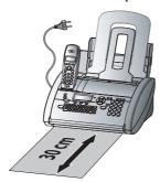
Avoid exposure to direct sunlight (the cartridge is heat-sensitive) and close proximity to heaters, radios and TV sets, air conditioning vents, dust, water and chemicals is not advised.
