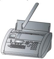
**2b** If you will be using the paper feeder constantly, flip the paper refill flap forwards and insert the paper holder in the appropriate holes behind the paper feeder. In this case, you can insert up to 50 sheets of paper.
