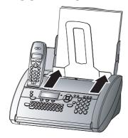
Never load paper while the fax machine is printing!
