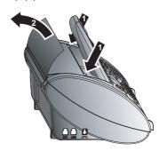
**2a** If you want to use the paper feeder for only a short while, flip up the paper support. In this case, you can insert up to 15 sheets of paper.
