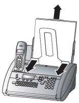
**2** Open the operation panel by lifting in the middle. When you hear a soft click, the panel is engaged.
